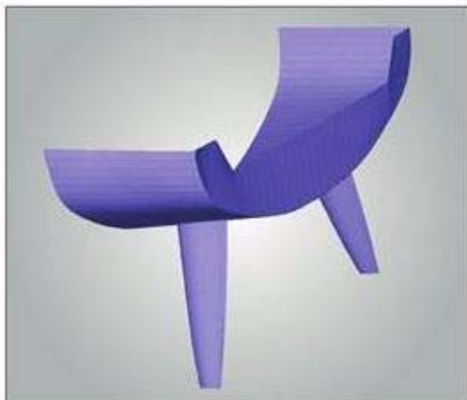
Many yachts requiring retrofitting do not have architectural designs available. Above —The laser scans provide remarkably precise measurements for the designers to work with. Right —OCD's redesign (in Maxsurf) of the same aft sections with new twin rudders.
