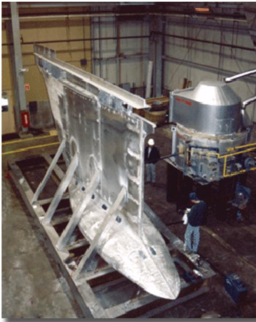
The problem was solved by casting the keel in Bridgeport. The logistics of moving one of our melt pots, the venting system, raw materials, and of course, the people to complete the pour was simply a matter of good planning and scheduling.
