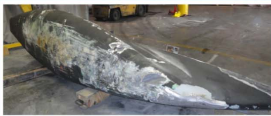
Hylas 70 in for grounding and keel bolt repair
