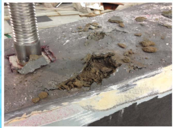
Exposed corrosion affect just under root cord
