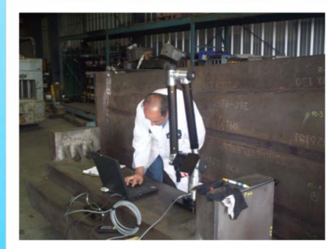
Inspection of rough fabrication by QC inspector, using a Faro Arm.
