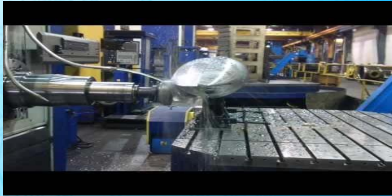
Custom cast retro bulb being CNC surfaced
