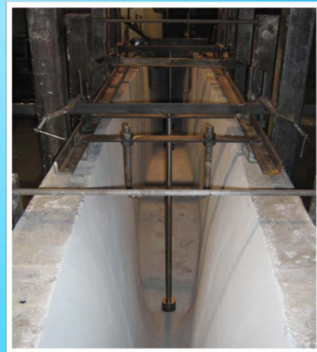
Typical two part ceramic mold, interior coated with release wash.
