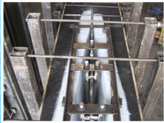
Typical sand mold, interior coated with mold release, blue- white colour
