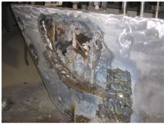
Opened frost bubble in side of keel
