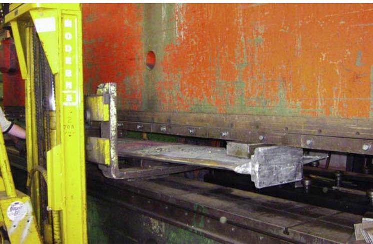
The team at MarsKeel has removed the keel and it is lying on it's side in the huge press where the twist and bend will be straightened.
