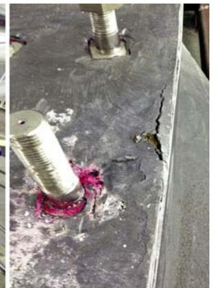
This is the keel off a 70 Hylas and the damaged barrier coating has allowed significant oxidation in the lead around the keel bolts.
