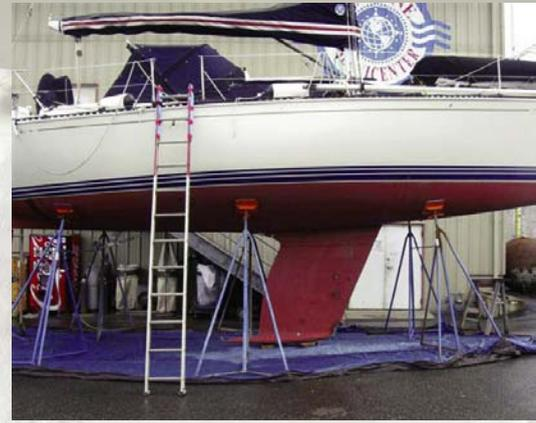
This CNC 34 suffered a whole list of problems including bent keel bolts, impact damage and a twist to its keel.
