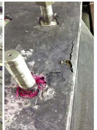
This is the keel off a 70 Hylas and the damaged barrier coating has allowed significant oxidization in the lead around the keel bolts.
