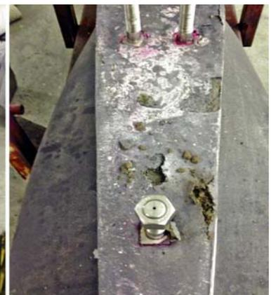
This shot is closer and reveals the oxidized lead looks like crumbly soil, not metal. The damage is extensive.
