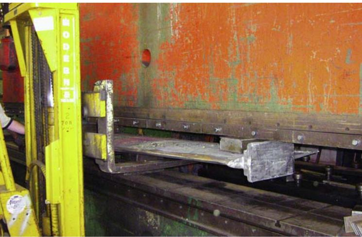
The team at MarsKeel has removed the keel and it is lying on it's side in the huge press where the twist and bend will be straightened.
