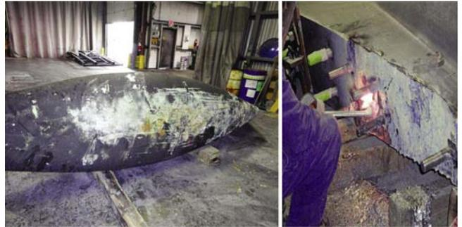
Now turned on its side, the experts at MarsKeel burn out the bad areas to replace the bolts and refuse new lead into the keel.
