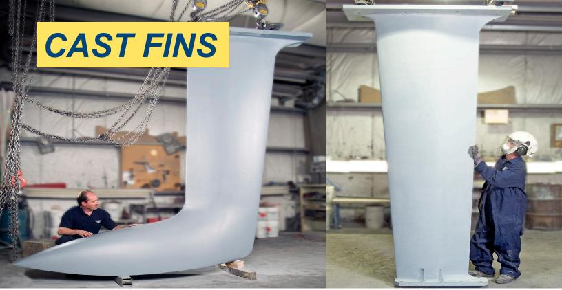
MarsKeel has produced cast keel fins and bulbs for such boats as Maxis Racing Yachts down to 6.5m Mini. The material range for the production of the fins goes from Nickel Aluminum Bronze to Grey Iron, Ductile Iron to 316 Grade to 2205 Duplex Stainless Steel. This combination of processes allows the customer to get a more complex fin shape and surface than can be produced through fabrication.
