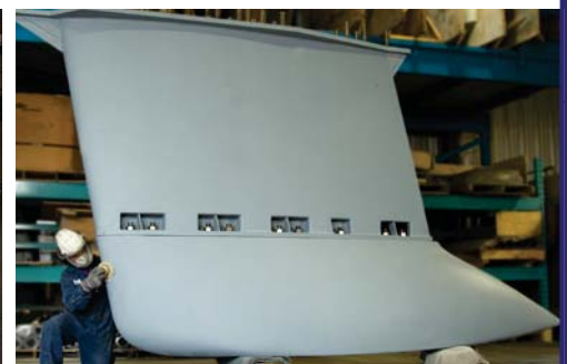
SWS 100 "L" fabricated fin dry fitted to cast bulb prior to disassemble and shipping.
