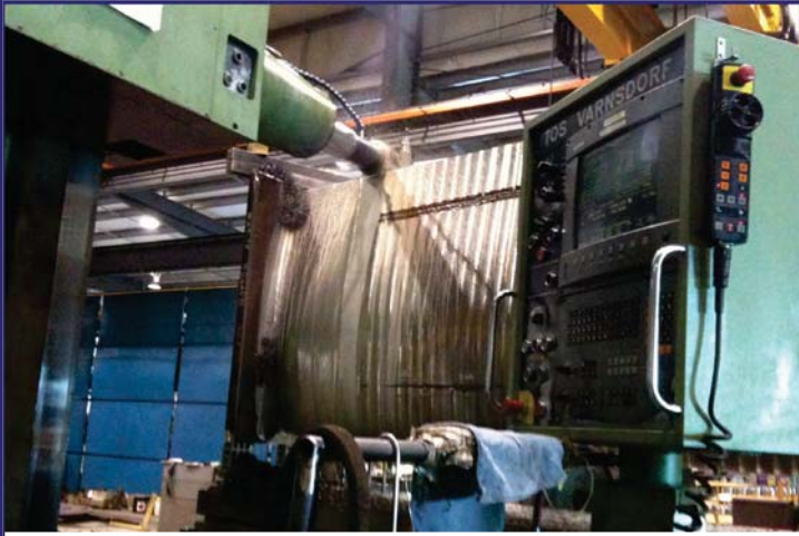
The SWS-9401 fin fabrication during the second surfacing pass on the horizontal CNC mill.
