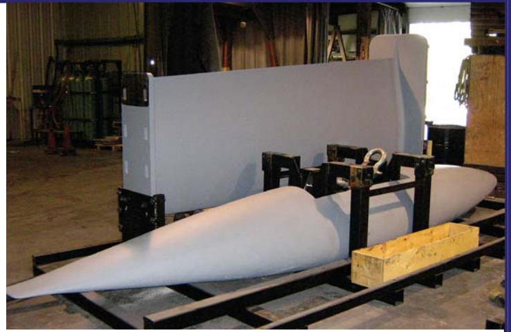
The completed SWS-9401 is dry fitted into a custom-made steel shipping cradle, prior to being loaded for shipment.
