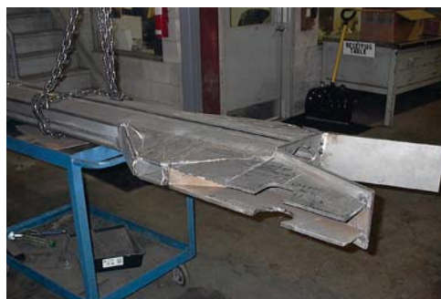
The internal structure of a 2205 Duplex lifting fin.
