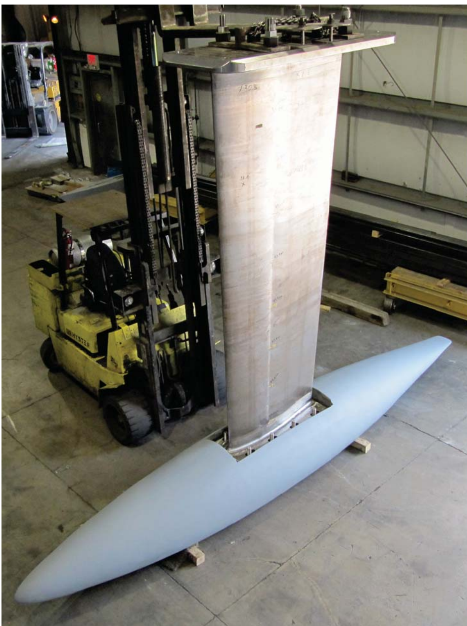
This is the dry fitting of SWS-9401 fin into its cast bulb, 32,000 lbs. The fin has just come off the mill, with no finish on it yet. This process is always done to ensure proper bolt alignment and all clearances are adequate for assembly by the customer, prior to shipment.
