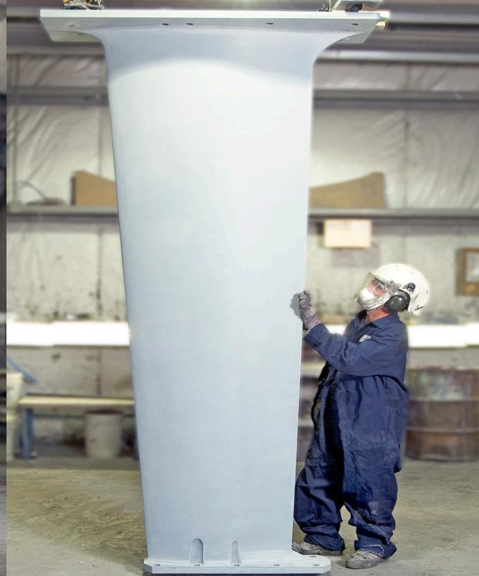
MarsKeel has produced cast keel fins and bulbs for such boats as Maxis Racing Yachts down to 6.5m Mini. The material range for the production of the fins goes from Nickel Aluminum Bronze to Grey Iron, Ductile Iron to 316 Grade to 2205 Duplex Stainless Steel. This combination of processes allows the customer to get a more complex fin shape and surface than can be produced through fabrication.
