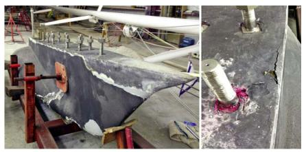
This is the keel off a 70 Hylas and the damaged barrier coating has allowed significant oxidization in the lead around the keel bolts.
