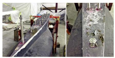
This shot is closer and reveals the oxidized lead looks like crumbly soil, not metal. The damage is extensive.
