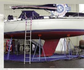
This CNC 34 suffered a whole list of problems including bent keel bolts, impact damage and a twist to its keel.
