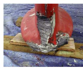
This is a closer shot of the bottom of the keel showing the area where the impact occurred.
